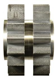
This is a picture of the spur gears used in the FZG test for gear scuffing. The left gear being a commercial gear product and the right gear being a gear protected with Champion's gear additive technology
